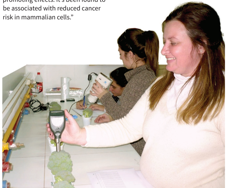
Agronomist Melina Buttarelli determines the firmness of the broccoli heads produced under pot conditions. Photo by Fernando Felipe Muñoz.
